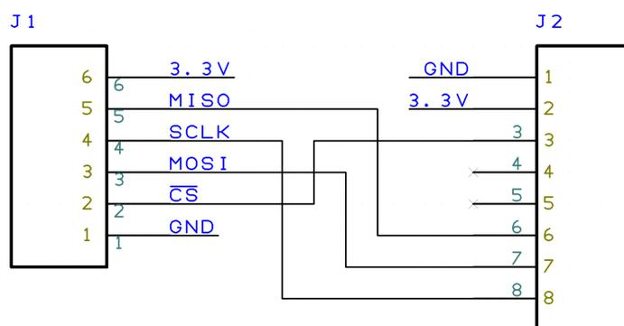
J1 is for USB-ISS and J2 is for the ADXL345 breakout board.
