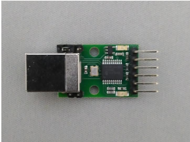
USB-ISS is a USB to Serial/I2C/SPI converter by Devantec, simple, small and easy to use. You don't need any extra library such as libusb and libftdi. Once plugged, the device is available on `/dev/ttyACM*` as a modem device.
