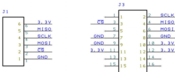
Minimum pins are used and each pin is directly corresponds to another's. Note that you only need to connect one of the power-line(3.3V and GND), because they are connected in the breakout board.
