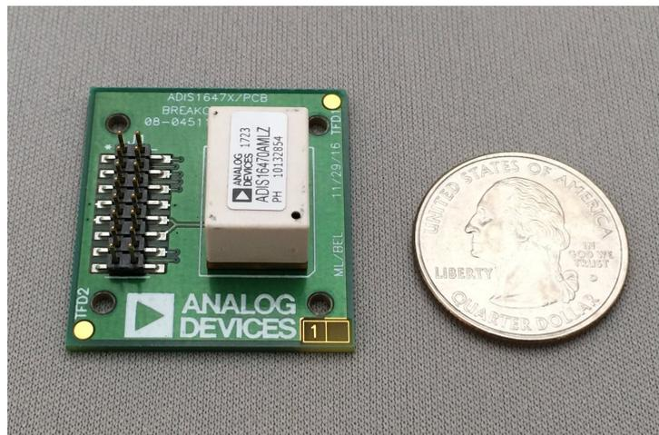
The sensor device is a BGA mounted chip, so it should be easier to use the breakout board. The following section assumes to use this breakout board.
