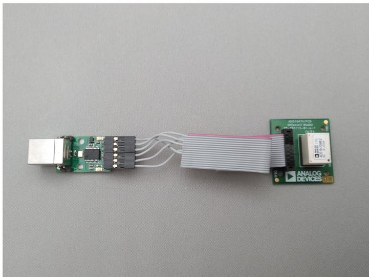
You need to build a flat cable to connect the USB-ISS and the ADIS16470 breakout board. The picture shows an implementation.
